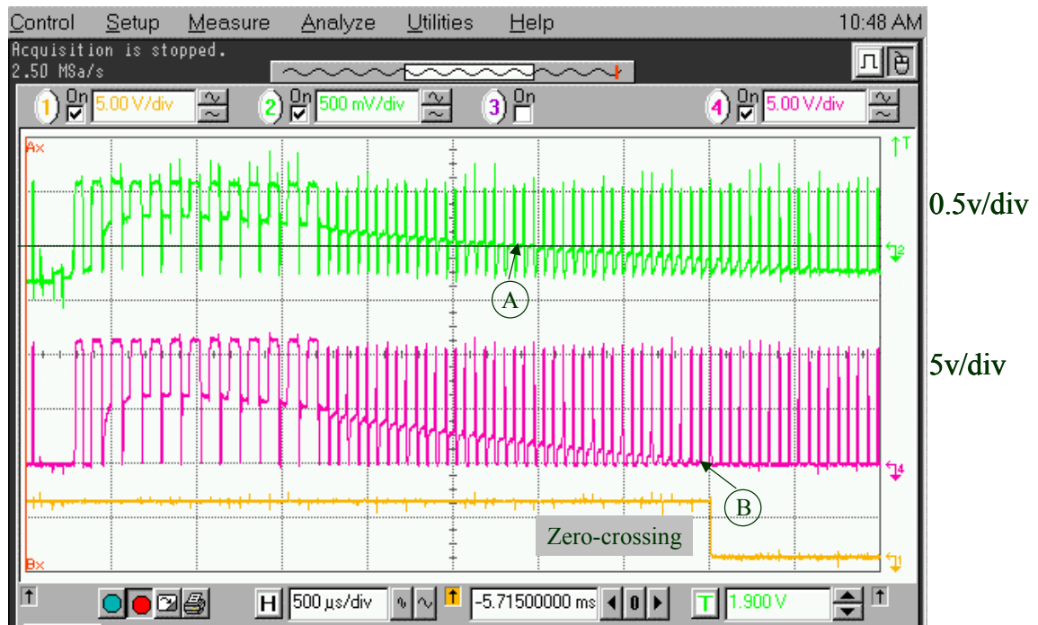
Fig.3.8 The upper channel: input signal to the pre-conditioning circuit; middle channel: output signal from the pre-conditioning circuit; lower channel: zero crossing detected.
